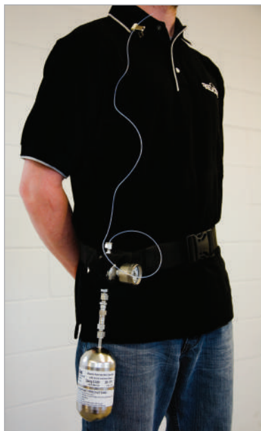
Sampling belt & personal sample inlet
